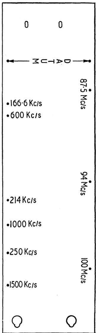
A dummy alignment scale, reproduced full size for use when calibrating the r.f. circuits
