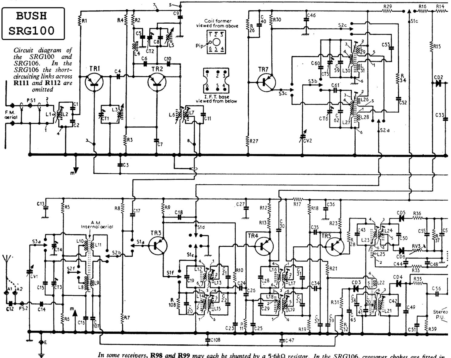
In some receivers, R98 and R99 may each be shunted by a 5-6kΩ resistor. In the SRG106, crossover chokes are fitted in.
