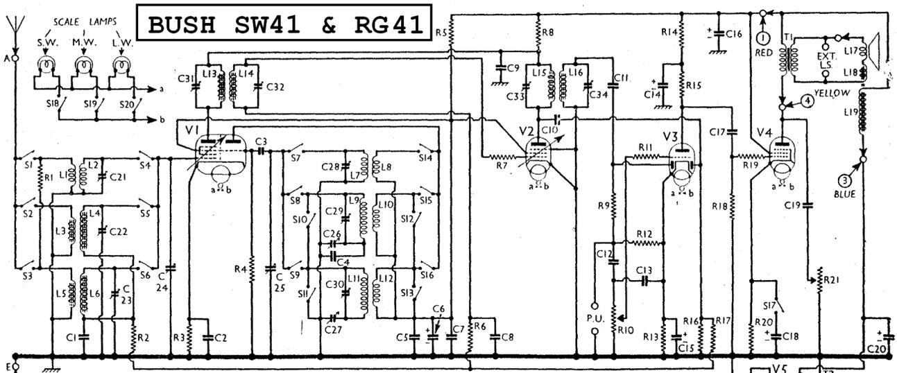
Circuit diagram of the Bush SW41 3-band superhet. The RG41 (A.C.) has a similar circuit, except for the inclusion of pick-up switching and one or two other modifications which are explained under "General Notes."
