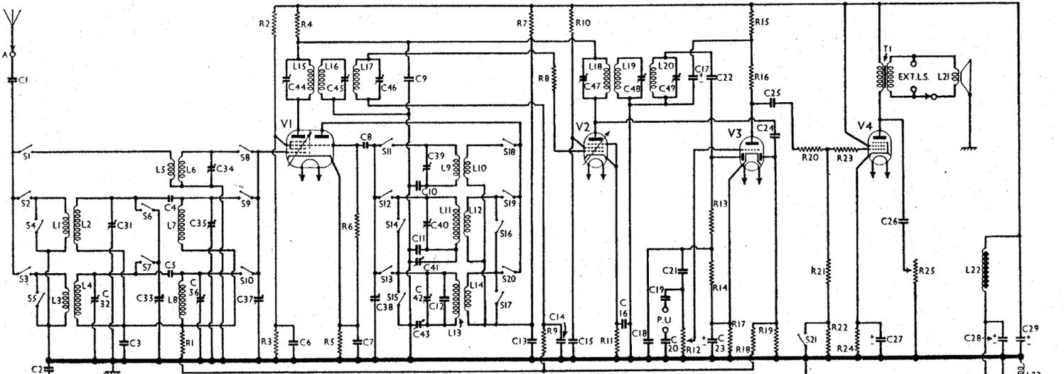
Circuit diagram of the Bush DAC43 3-band superhet for A.C. or D.C. mains. The RG43 radiogram has a somewhat similar chassis, the modifications being noted on page V. A metal rectifier is used for the H.T. supply when the set is working on A.C.
