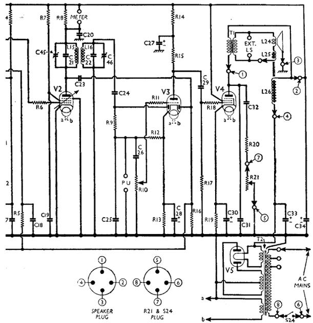
is "out," the associated a and b switches are open, and the x switches closed. When a button is "in," its a and b switches are closed and its x switches are open.
