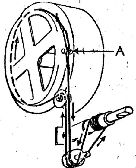
Remove **R18** temporarily, set the gang to minimum capacitance, turn the control spindle to its stop in an anti-clockwise direction, slip the loop over the small stud **A**, seen in the sketch, and wind the cord in the direction shown there. Make six turns round the spindle, but do not permit one turn to overlap another.
