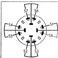
Diagram of the wave band switch unit, as seen from the rear. SX is found only in later chassis.
