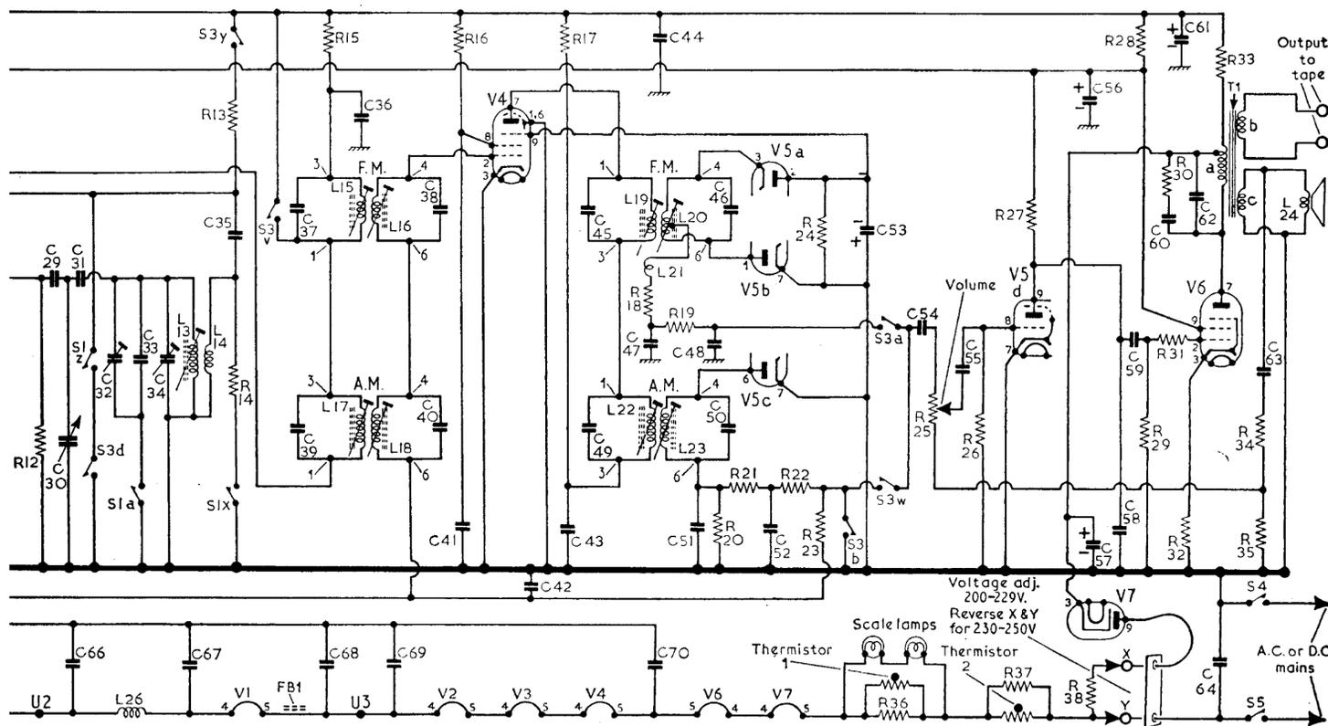
**Equipment Required.**—An amplitude modulated signal generator covering the A.M. alignment frequencies 200-1,500kc/s and the F.M. alignment frequencies 10.7Mc/s and 87.5-100Mc/s; an audio output meter to match a 3Ω impedance; a Model 8 Avometer or D.C. valve voltmeter for use as a D.C. output meter; a 0-50μA microammeter; two matched 47kΩ resistors; a 1kΩ resistor for use as a damping shunt; a 0.1μF capacitor; and a non-metallic screwdriver-type trimming tool.
