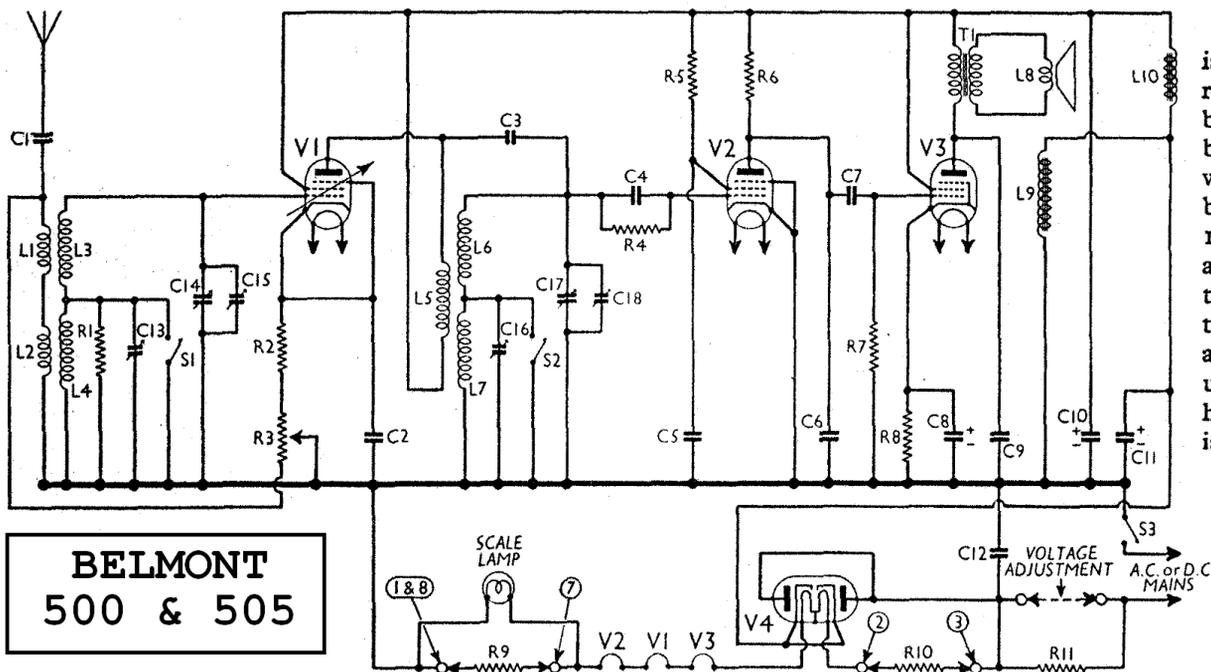
**R11** is the line cord resistor, and can be shorted out by a 2-pin plug when the set is to be used on 100-110 V mains. **R9** and **R10** are in the K52H resistance tube, and a diagram of the underside of the holder of this is below the circuit.
