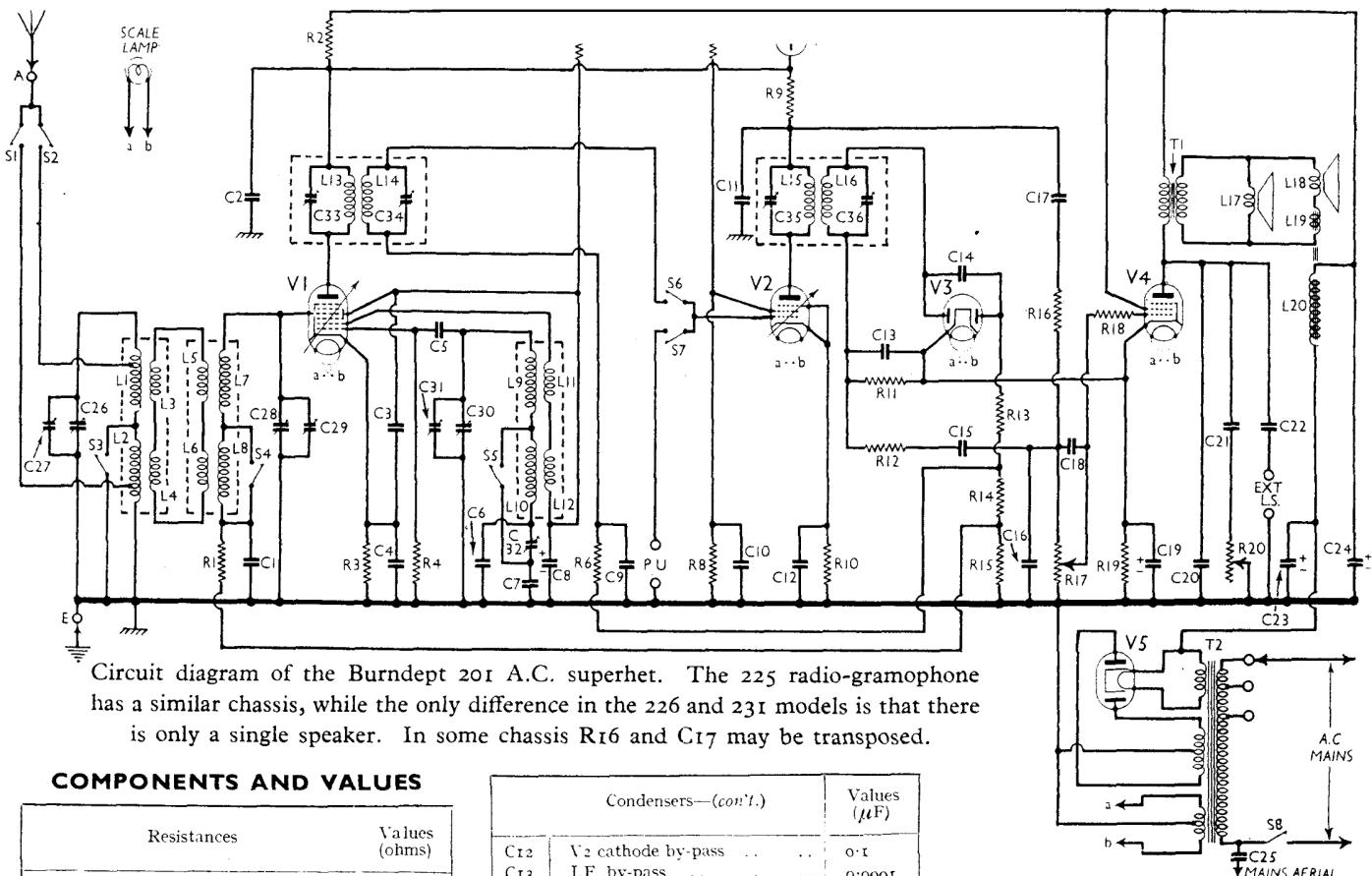
Circuit diagram of the Burndept 201 A.C. superhet. The 225 radio-gramophone has a similar chassis, while the only difference in the 226 and 231 models is that there is only a single speaker. In some chassis R16 and C17 may be transposed.
