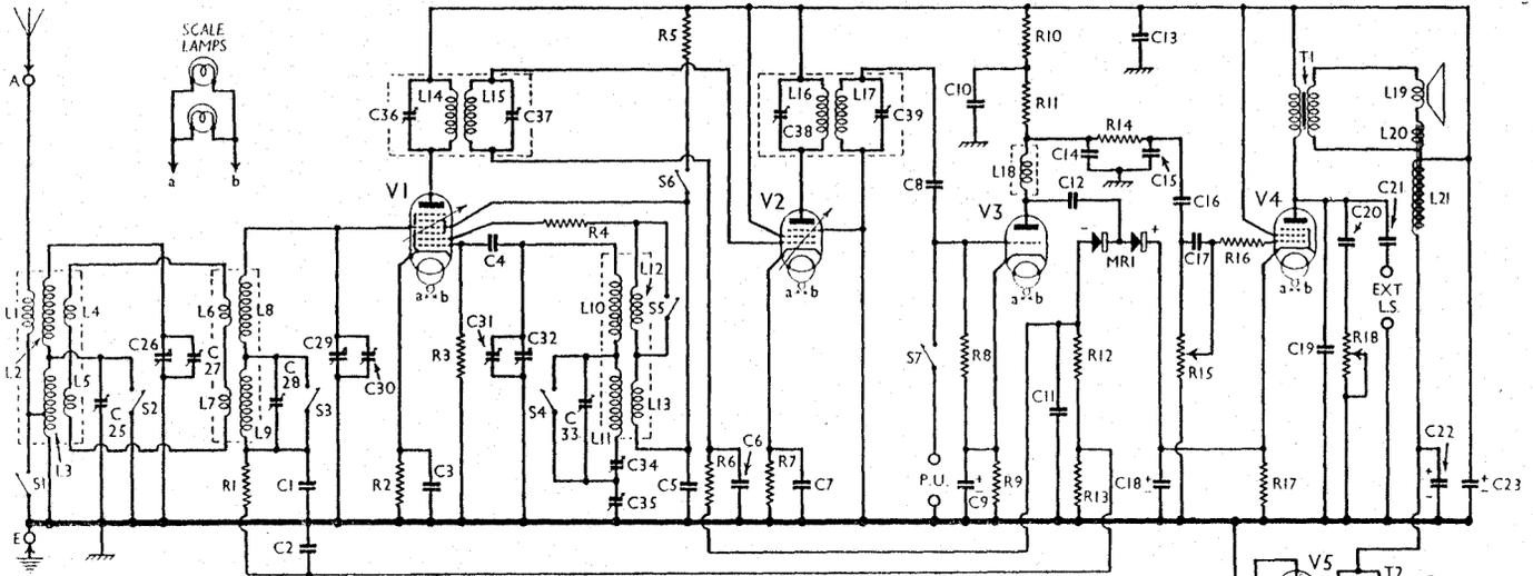
Circuit diagram of the Burndipt 257 A.C. superhet. Note that a Westector (MR1) is used for A.V.C. Early chassis may have a resistance in the control grid circuit of V1, while C2 may be omitted. S8 opens and mutes radio when the set is switched to Gram.
