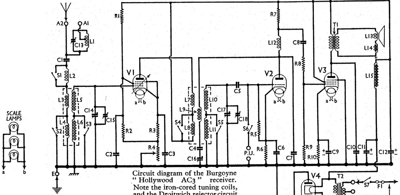
Circuit diagram of the Burgoyne "Hollywood AC3" receiver. Note the iron-cored tuning coils, and the Drotwisch retractor circuit
