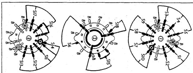
Switch diagrams, looking at the units in the directions of the arrows
