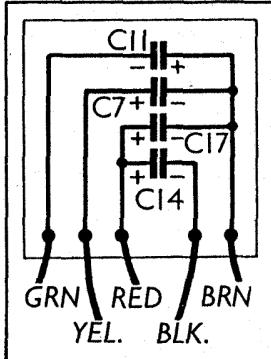
Diagram of the internal connections of the condenser block, with the colour coding of the leads.
