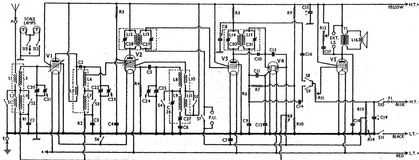
An indirectly heated double diode is used in the Alba 230 battery superhet, and although the I.F. valve is a variable-mu type, it operates with fixed bias. A.V.C. delay voltage is obtained from the potentiometer formed by R9 and R10.
