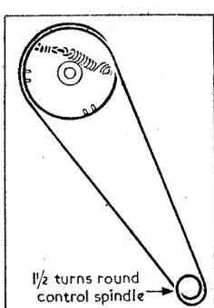
*Above:* Sketch of the tuning drive system as seen with the gang at minimum capacitance.
