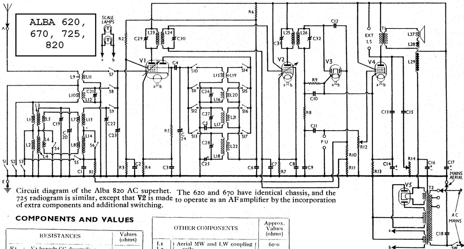
Circuit diagram of the Alba 820 AC superhet. The 620 and 670 have identical chassis, and the 725 radiogram is similar, except that V2 is made to operate as an AF amplifier by the incorporation of extra components and additional switching.
