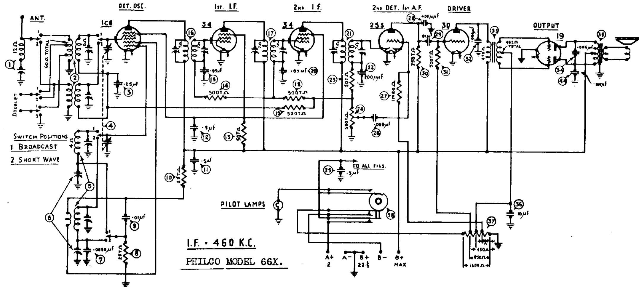
TYPE CIRCUIT : Battery operated, 6 valve, dual wave superheterodyne using A.V.C.
