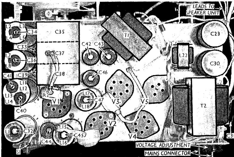
Plan view of the chassis. All the trimmers are indicated here, many of them in the tops of their coil cans. R<sub>2</sub> is carried in the top cap connector of V<sub>1</sub>.
