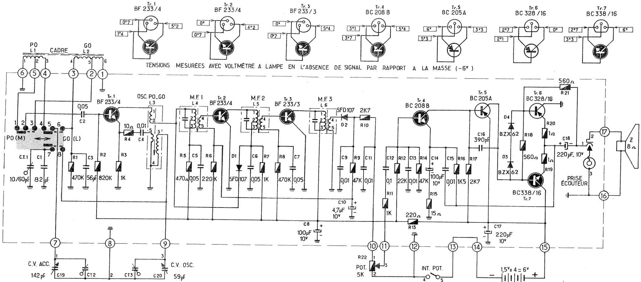
TENSIONS MESURÉES AVEC VOLTMÈTRE A LAMPE EN L'ABSENCE DE SIGNAL PAR RAPPORT A LA MASSE (-6V)
