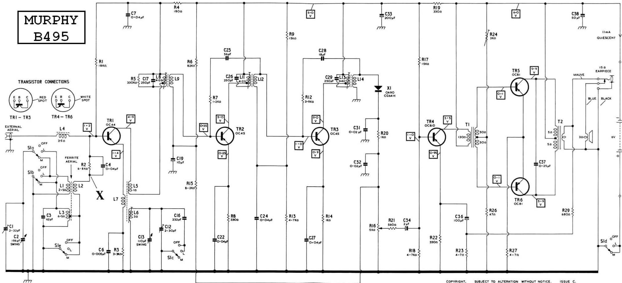
The wave-range switch is shown in the M position. Circuit voltages are shown within rectangles and were measured on the M range under no-signal conditions using a 20,000
