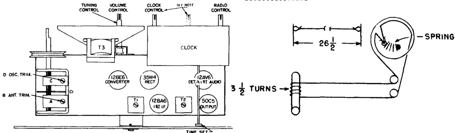
NOTE: SOME CHASSIS WILL INCLUDE CLOCKS USING THREE KNOBS; LABELED AS FOLLOWS: ALARM CONTROL, SLEEP CONTROL AND RADIO CONTROL.
