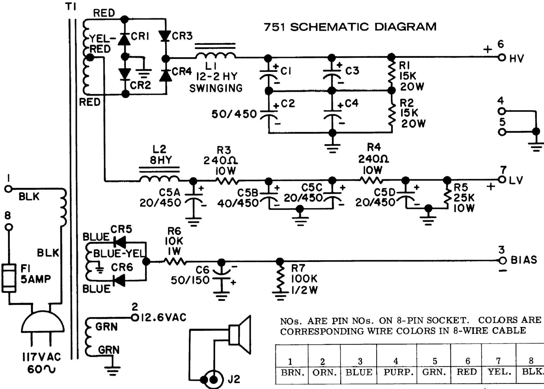
NOs. ARE PIN NOs. ON 8-PIN SOCKET. COLORS ARE CORRESPONDING WIRE COLORS IN 8-WIRE CABLE
