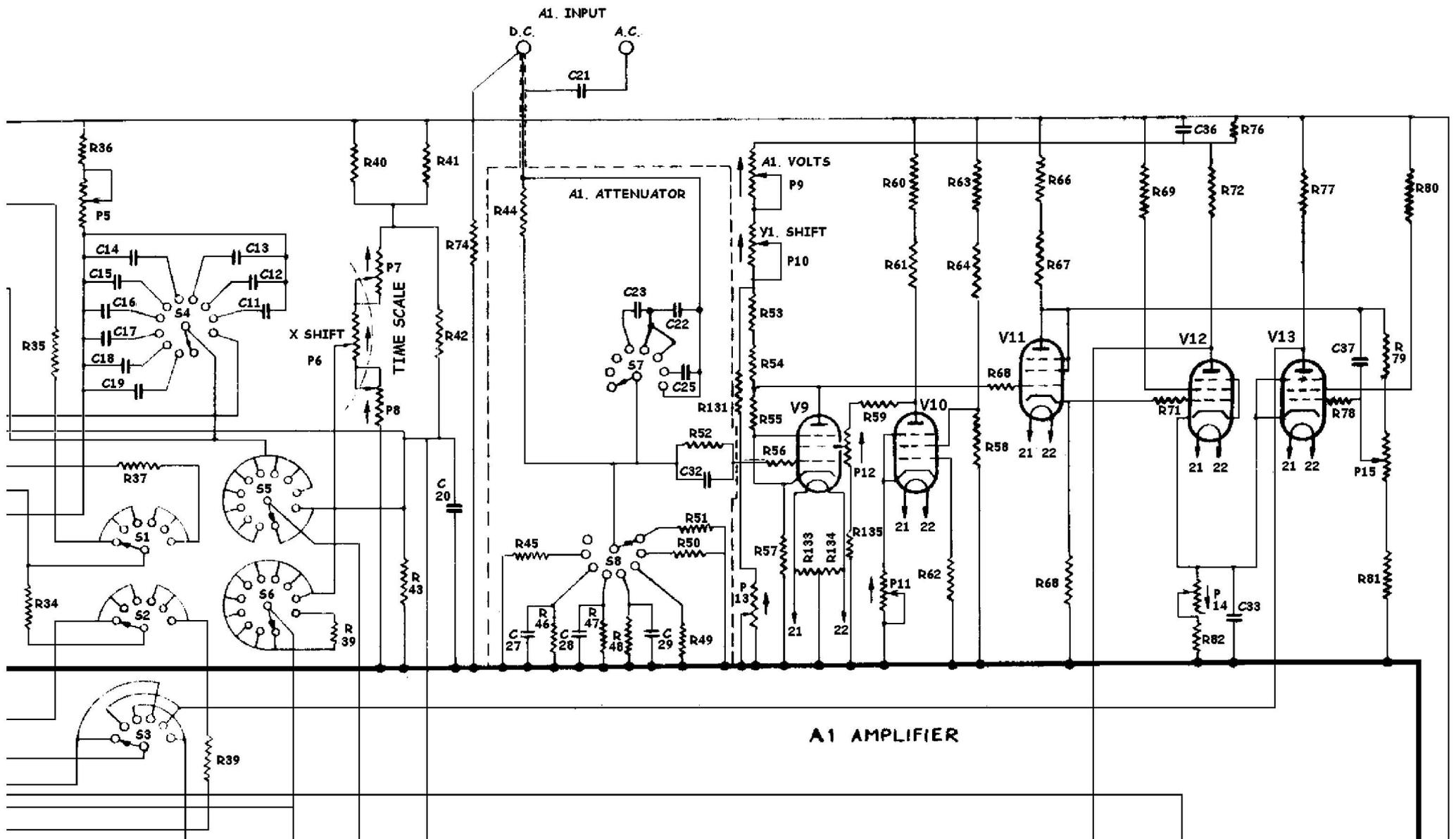
Cossor Model 1049 Double Beam Oscilloscope
