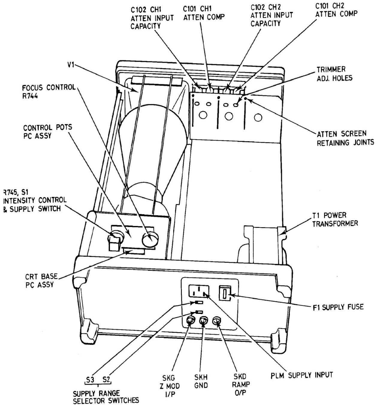
Fig. 3 Internal Assembly – bottom view
