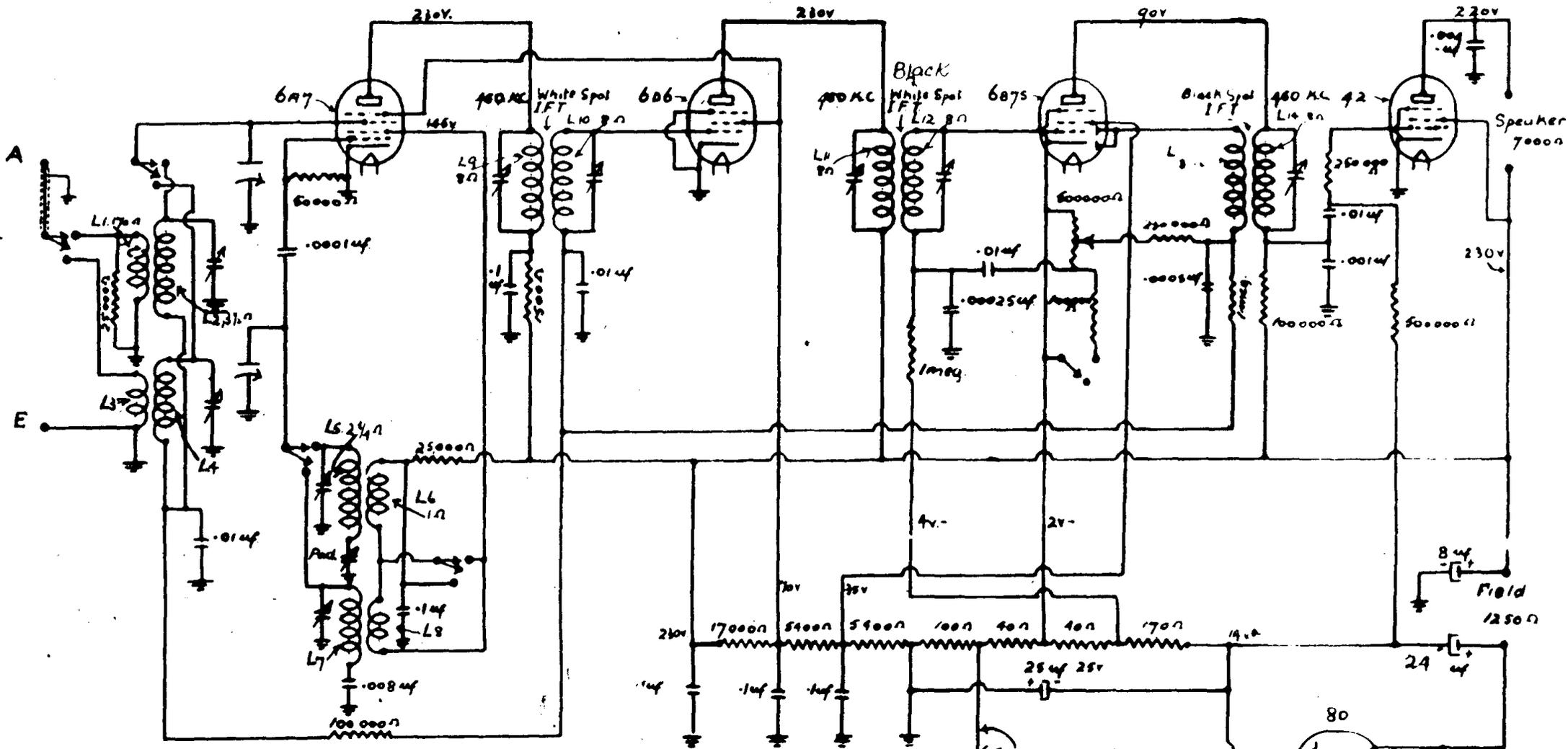
Coils L1, L2, L7, L8 Comprise White Spot Coil
