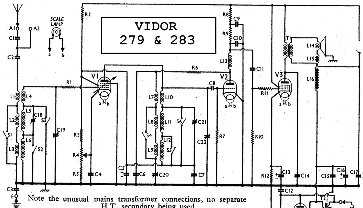
Note the unusual mains transformer connections, no separate H.T. secondary being used.
