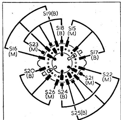
Diagram of the mains/battery change-over switch unit, drawn as seen from the front of the chassis, after removal from the carrying case. The suffixes (B) and (M) indicate that the switches close on battery and mains respectively.
