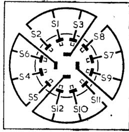
**L.W.**—Switch receiver to L.W., disconnect signal generator leads from **A** and **E** sockets and lay them near the carrying case. Tune receiver to "Paris" on L.W. scale, feed in a 1,829 m (164 kc/s) signal and adjust the cores of **L8** (B1) and **L5** (A2) for maximum output. Tune to "Kalundborg" on scale, feed in a 1,224 m (245 kc/s) signal and adjust **C38**
