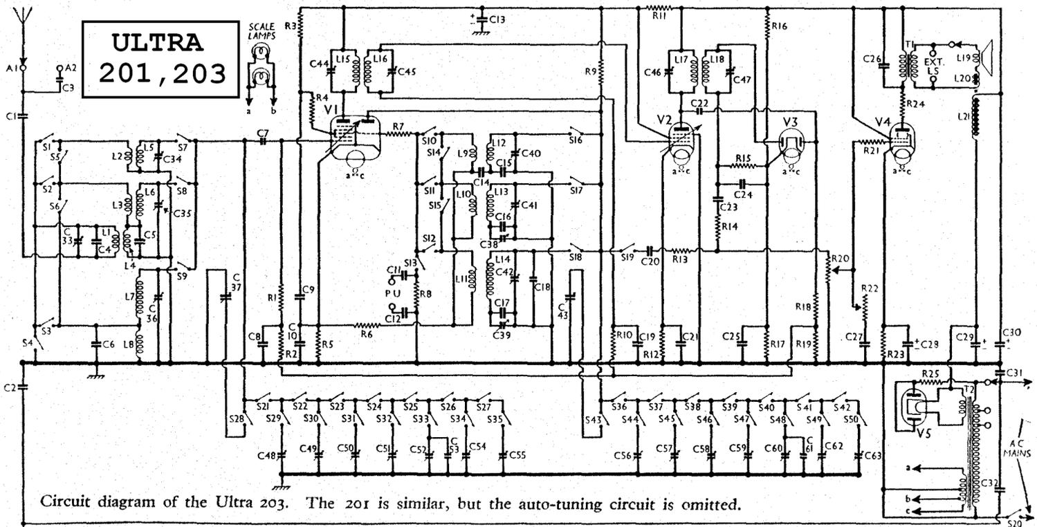
Circuit diagram of the Ultra 203. The 201 is similar, but the auto-tuning circuit is omitted.
