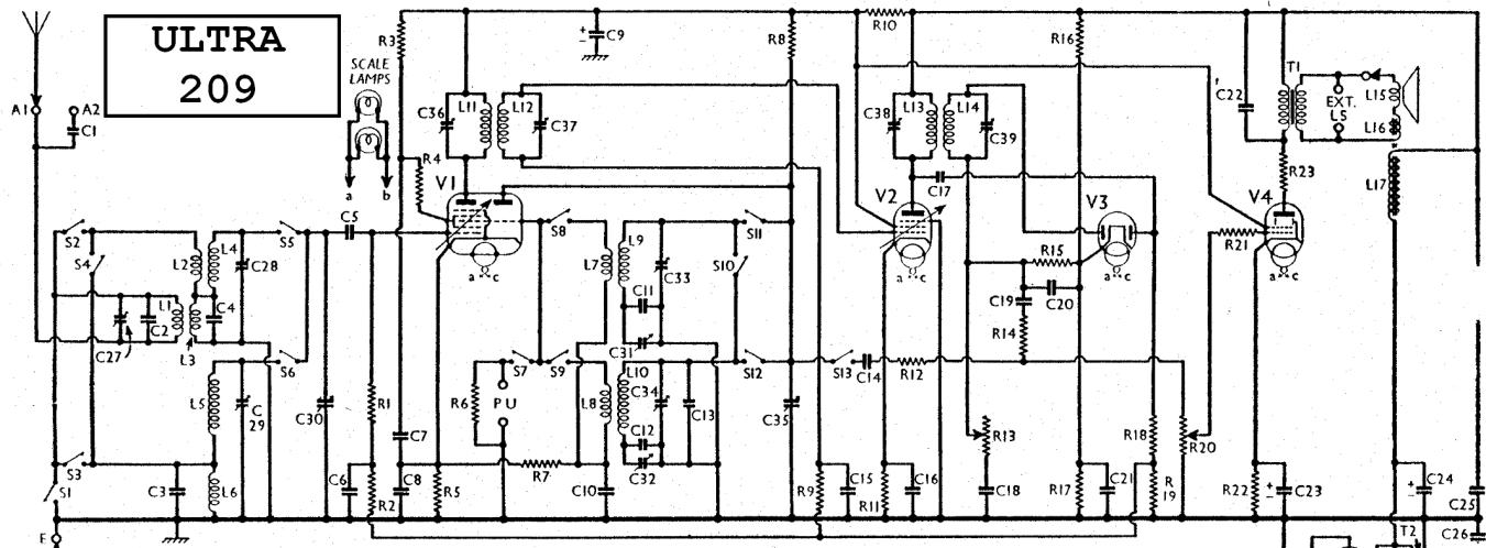
Note the IF rejector circuit **L1**, **C2** and **C27**, the loading circuits **L3**, **C4** and **L6**, **C3** which provide a special form of aerial coupling, and the arrangements for a pick-up whereby the triode section of **V1** is used as an AF amplifier.
