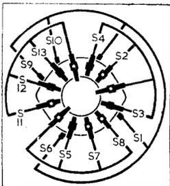
Diagram of the waveband switch unit, as seen from the rear. Below is the associated switch table.
