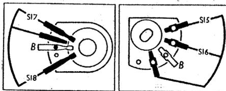
*Left.*—Diagram of the speaker circuit switch unit S17, S18 drawn as seen from the under side of a chassis standing on its back. *Right.*—Diagram of the tone control switch unit S15, S16, drawn as seen from the rear of an inverted chassis. B indicates a blank tag.
