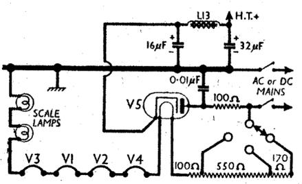
Mains input and power supply circuit in the A.C./D.C. models. The values of added components are indicated. The lowest tapping on the ballast resistor is for .100V mains.
