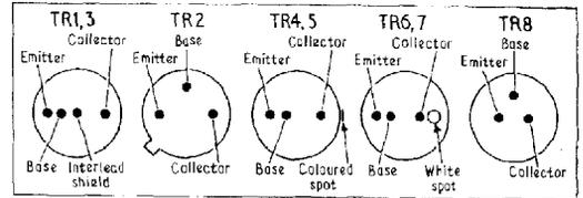
Above: Transistor terminal connections
