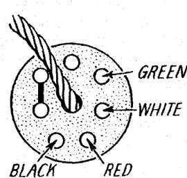
Plan diagrammatic view of the speaker plug, showing the colour coding of the wires to the pins.
