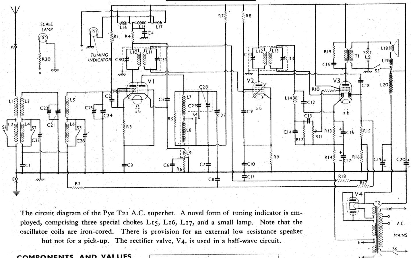
The circuit diagram of the Pye T21 A.C. superhet. A novel form of tuning indicator is employed, comprising three special chokes L<sub>15</sub>, L<sub>16</sub>, L<sub>17</sub>, and a small lamp. Note that the oscillator coils are iron-cored. There is provision for an external low resistance speaker but not for a pick-up. The rectifier valve, V<sub>4</sub>, is used in a half-wave circuit.
