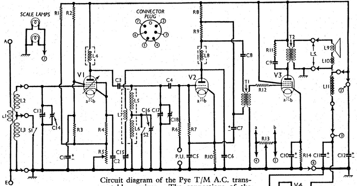
Circuit diagram of the Pye T/M A.C. transportable receiver. The connections of the power unit plug are indicated by numbered arrows, and of the power unit socket by correspondingly numbered circles. The other arrows and circles indicate frame aerial, speaker, and similar connections. A numbered diagram of the plug (or socket), viewed from the underside, is also given.
