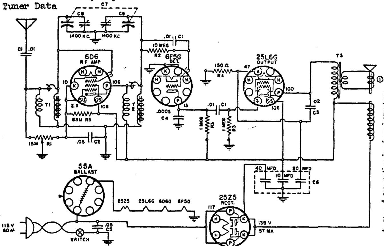
A ground connection is of no importance and therefore has been eliminated WHERE NO VOLTAGE READING IS SHOWN AT SOCKET PRONGS, IT INDICATES ZERO VOLTAGE OR A VERY LOW READING. ALIGNMENT IS TO BE MADE AT THE FREQUENCIES SHOWN AT THE TRIMMER CONDENSERS. CAPACITY VALUES ARE IN MICROFARADS.
