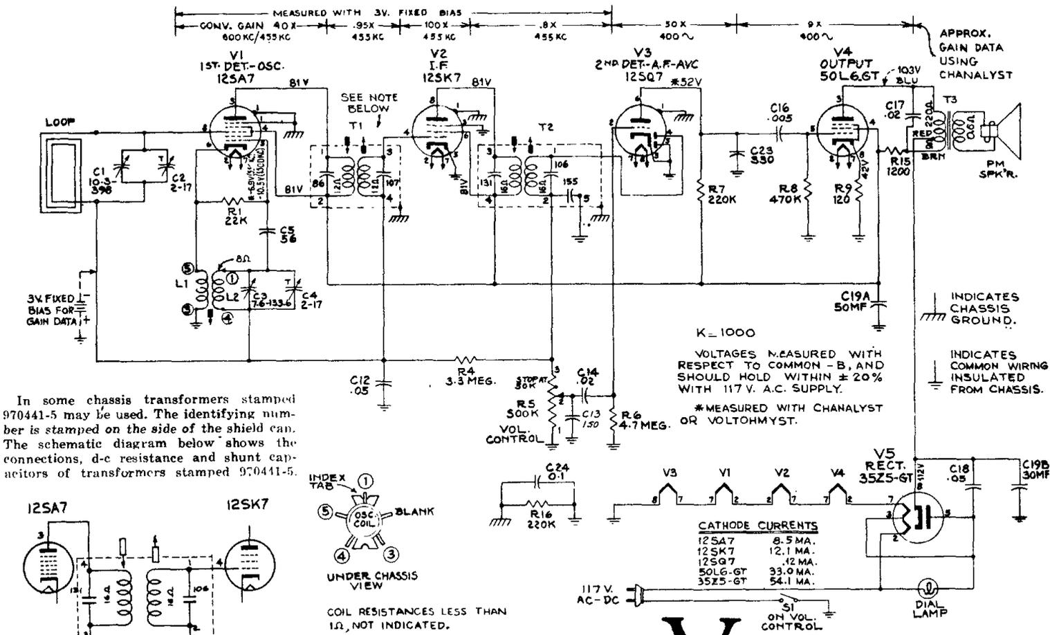
In some chassis transformers stamped 970441-5 may be used. The identifying number is stamped on the side of the shield can. The schematic diagram below shows the connections, d-c resistance and shunt capacitors of transformers stamped 970441-5.
