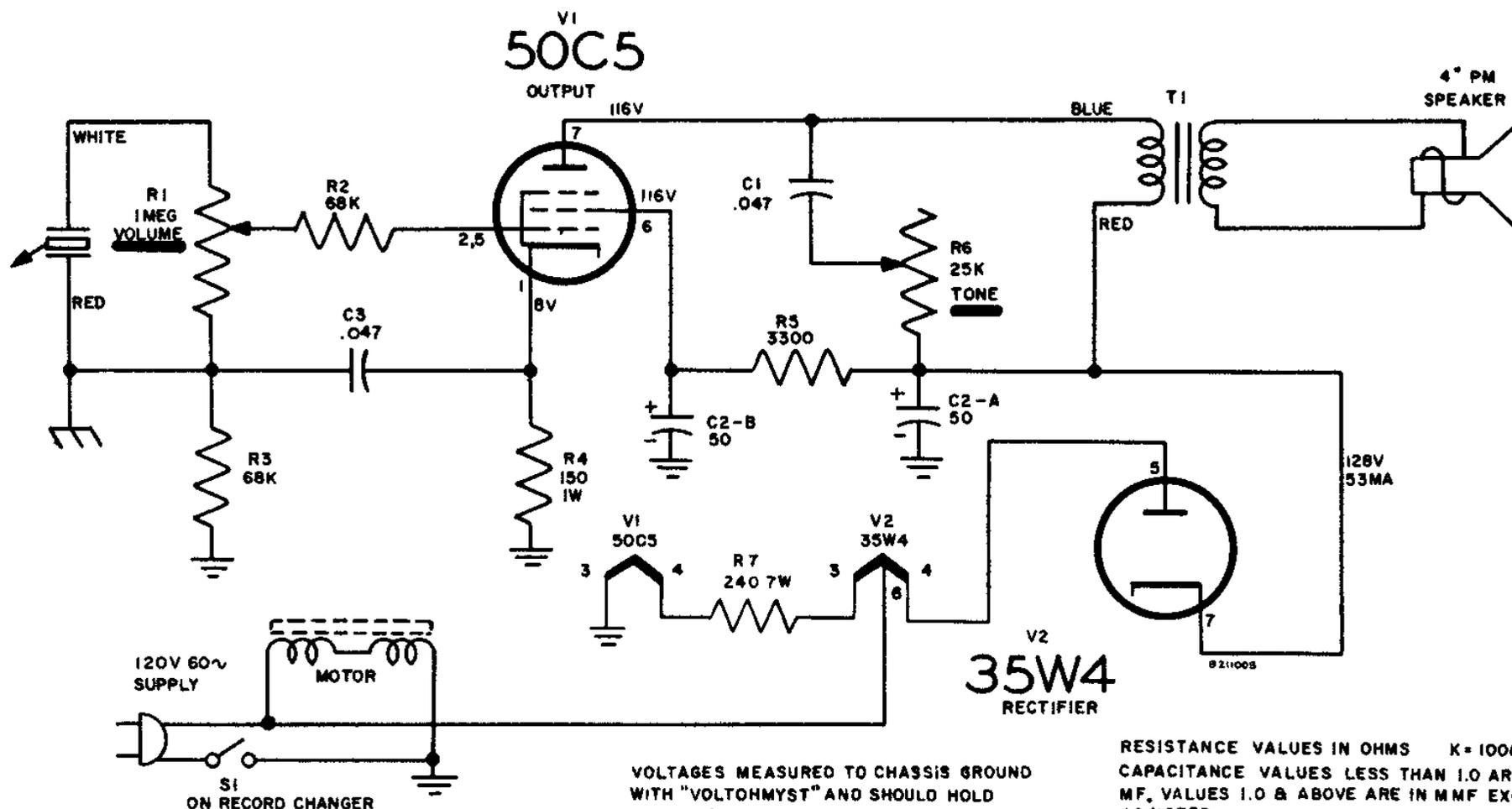
VOLTAGES MEASURED TO CHASSIS GROUND WITH "VOLTOHMYST" AND SHOULD HOLD WITHIN  $\pm 20\%$  WITH RATED LINE VOLTAGE.
