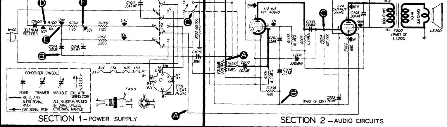
**OSCILLATOR TEST** Connect the positive lead of a high-resistance voltmeter to test point D; connect the prod end of the negative lead through a 100,000-ohm isolating resistor to the oscillator grid (pin 1 of the 1R5), test point C. Use a suitable meter range, such as 0-10 volts. Proper operation of the oscillator is indicated by negative voltage within the range given in the chart (measured with a 20,000-ohms-per-volt meter) throughout the tuning range.
