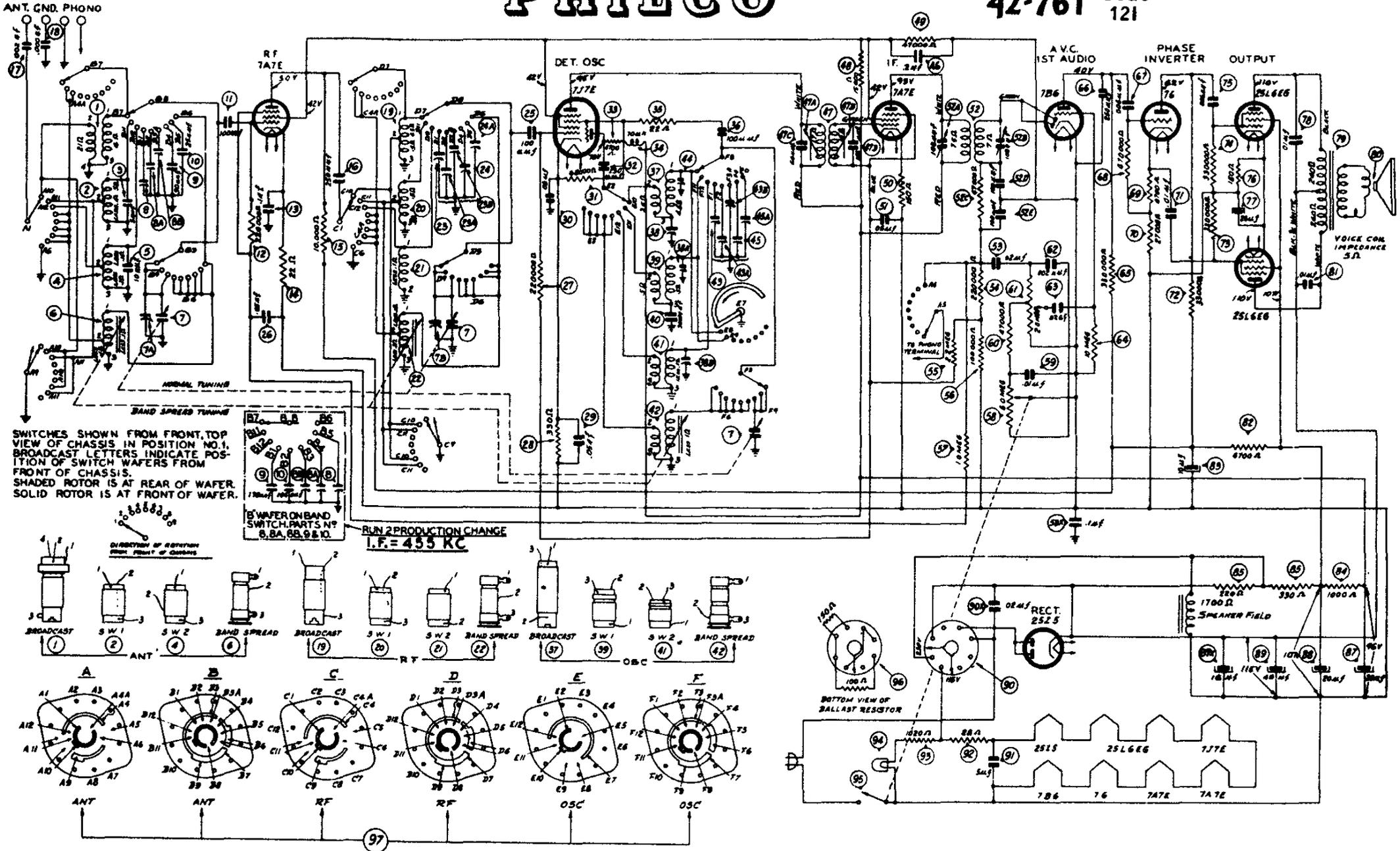
The voltages indicated at the tube elements above were measured with a 1000 ohms per volt voltmeter. Philco Model 027, line voltage 117 volts, A. C. band switch (broadcast). No station being received.
