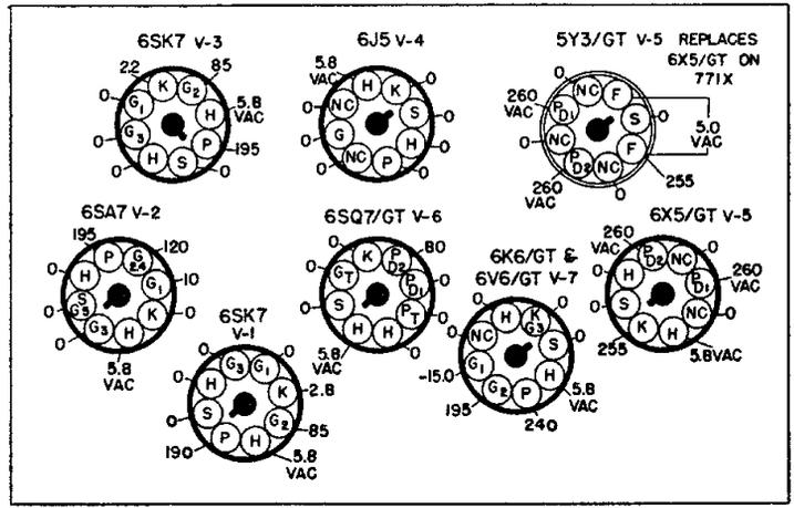
All D.C. voltages measured with a vacuum tube voltmeter from socket contacts to chassis.—A.C. voltages measured with a 1000 ohms per volt A.C. meter from socket contacts to chassis.
