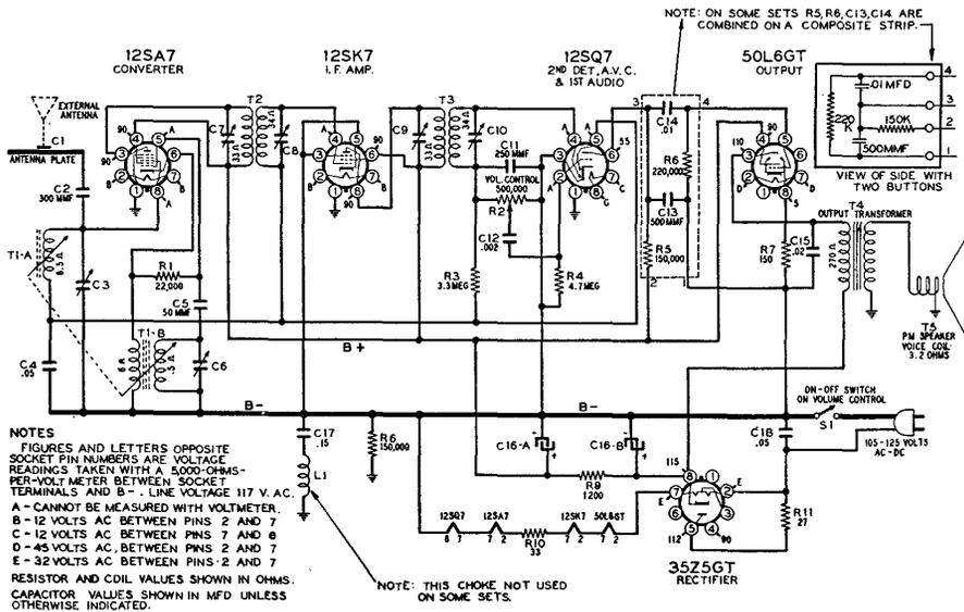
NOTES: On some sets dual trimmer C3, C6 is grounded to chassis instead of to B- as shown above. On some sets R6 is 470K ohms and R5 is 220K ohms. On some sets R10 is not used.
