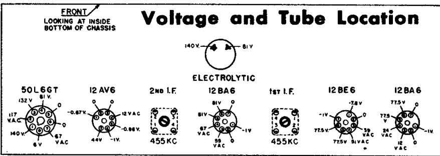
Measurements are made at 117V line, using electronic Voltmeter. Except where otherwise indicated, voltages are D.C. and are positive with respect to the reference point which is the common Black-White lead.
