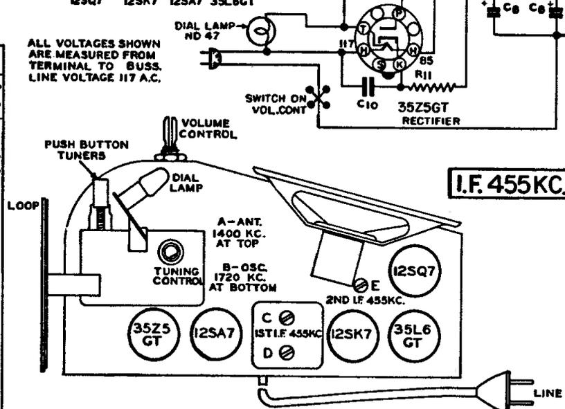
**GENERAL DATA.** The alignment of this receiver requires the use of a test oscillator that will cover the frequencies of 455, 600, 1400 and 1720 KC and an output meter to be connected across the primary or secondary of the output transformer. If possible, all alignments should be made with the volume control on maximum and the test oscillator output as low as possible to prevent the AVC from operating and giving false readings.
