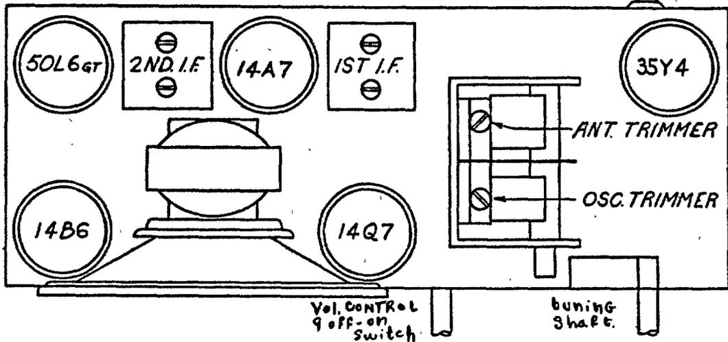
Remove chassis from cabinet for alignment.
