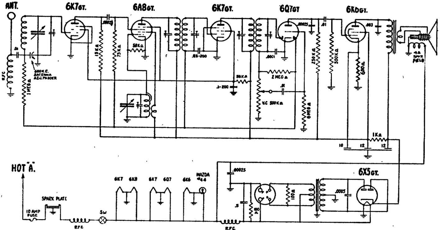
**I. F. ALIGNMENT** Set the variable condenser at minimum capacity, (dial pointer at 1550 K.C.). Connect the two leads from a good, modulated signal generator, the ground lead to the radio chassis and the other lead through a .1 mfd. condenser, to the grid cap of the 6A8GT with the tube's grid lead still in place.
