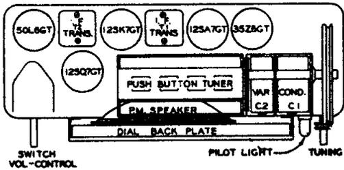
Tuning range 540 Kc to 1600 Kc. Intermediate frequency—455 Kc. RF and IF measurements made at 50 milliwatts output—approximately .38 volt on a rectifier type voltmeter connected across the voice coil.
