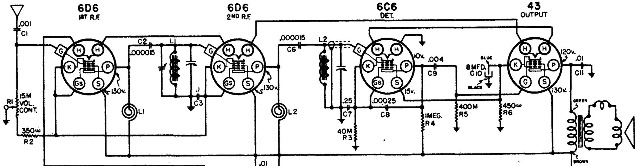
TUBE SOCKETS ARE VIEWED FROM UNDER SIDE OF CHASSIS. VOLTAGE READINGS AT INDICATED SOCKET PRONGS ARE TO CHASSIS. ALIGNMENT IS TO BE MADE AT THE FREQUENCY SHOWN AT THE TRIMMER CONDENSER. WHERE NO VOLTAGE READING IS SHOWN AT SOCKET PRONG, IT INDICATES A VERY LOW READING. VOLUME CONTROL TO BE ON FULL.
