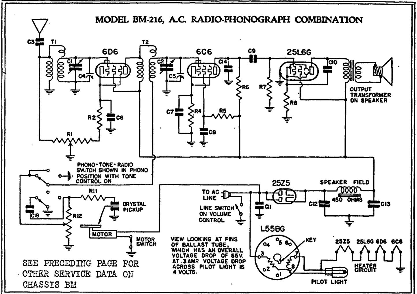
**Caution:** The motor used in this combination is of the synchronous type and will operate on **ALTERNATING CURRENT ONLY**. To avoid damaging the motor, the combination should never be used on direct current.
