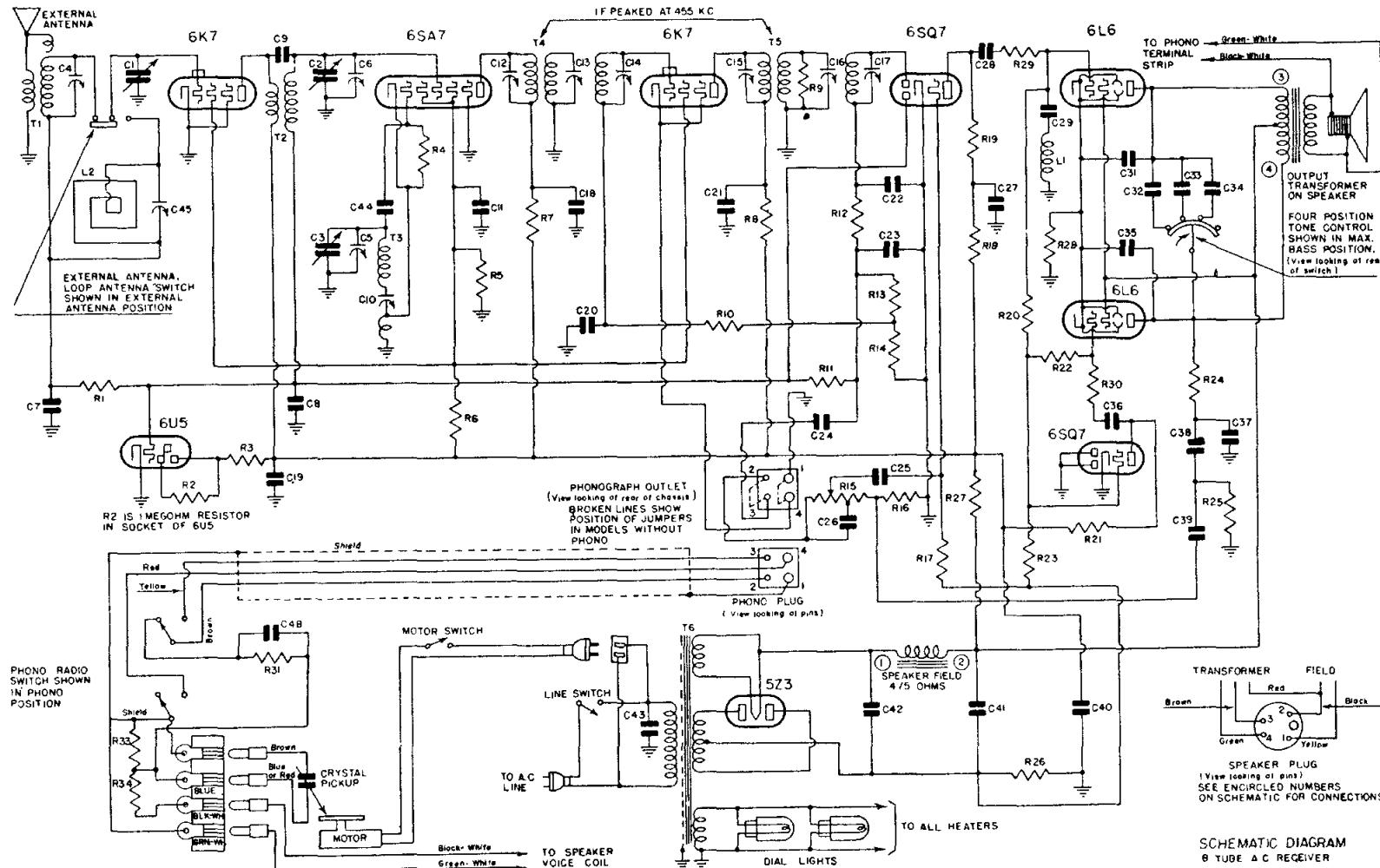
Readings should be taken with a 1000 ohms-per-volt meter. Voltages listed below are from point indicated to ground (chassis) with the volume control turned on full and no signal. Line voltage for these readings was 117 volts, 60 cycles, a.c. All readings except B plus at rectifier, heaters, and cathode voltages were taken on 300 volt scale.
