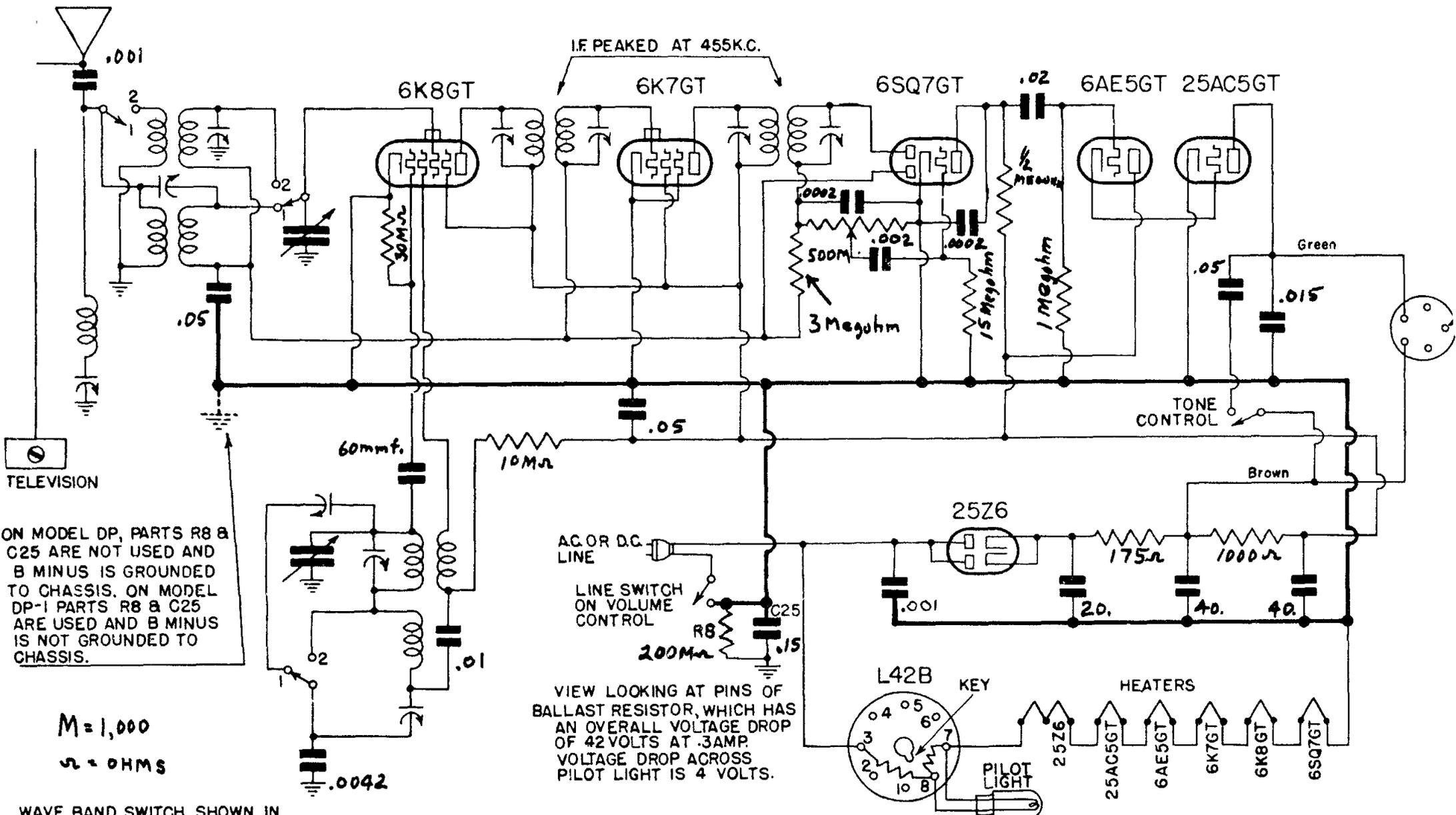
ON MODEL DP, PARTS R8 & C25 ARE NOT USED AND B MINUS IS GROUNDED TO CHASSIS. ON MODEL DP-1 PARTS R8 & C25 ARE USED AND B MINUS IS NOT GROUNDED TO CHASSIS.
