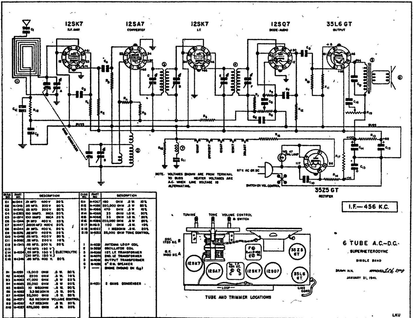
Voltages shown on the circuit diagram are from socket terminals to ground buss. In measuring voltages use a voltmeter having a resistance of at least 1000 ohms per volt. Allowances should be made for variations in line voltage.
